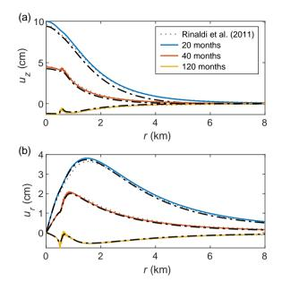
**Figure 7.** Radial distribution of the vertical (a) and horizontal (b) ground displacement at sequential times. The coloured and dash-dotted lines correspond to methods A and B, respectively.
