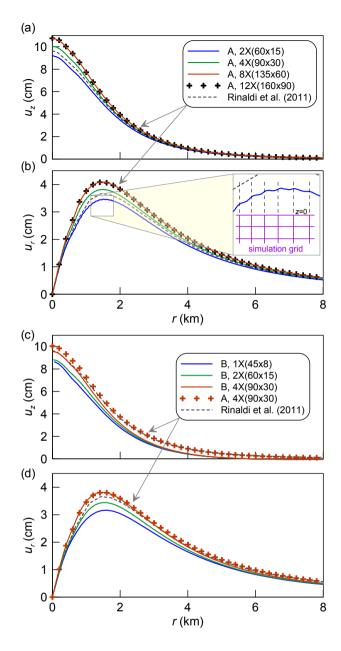
Figure 8. Displacements  $u_z$  (a and c) and  $u_r$  (b and d) at t = 20 months calculated using different methods and grids. The oscillatory behaviour of u shown in panel (b) is caused by the space discretisation.
