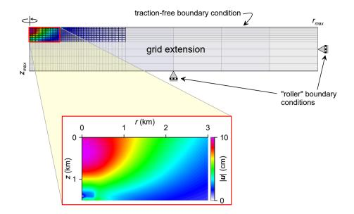
Figure 5. The domain and the boundary conditions for the geomechanical simulation by method B. The mesh used for the fluid flow modelling is shown in black. The distribution of total displacement is shown at t = 20 months.
