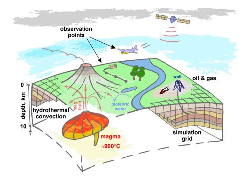
**Figure 1.** Sketch of typical processes in hydrothermal systems (left) and petroleum reservoirs (right). Magma degassing results in a plume of hot magmatic fluid. Near the surface, the fluid can mix with colder meteoric water. The observation points, where the ground displacement and gravity changes can be measured, are shown.
