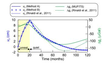
Figure 6. Vertical components of the ground displacement  $(u_z)$  and gravity change  $(\Delta g_z)$  at the centre OP (r = 0, z = 0) against time.
