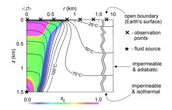
Figure 4. The simulation domain and the boundary conditions for the hydrodynamic simulation. The distribution of the gas saturation  $(s_g)$  and the isotherms are shown at t = 120 months.
