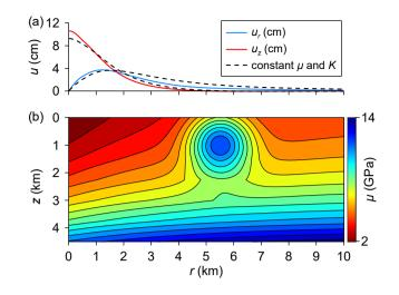
Figure 9. Distributions of  $u_r$  and  $u_z$  at z = 0 km and t = 20 months (a) and shear modulus (b).
